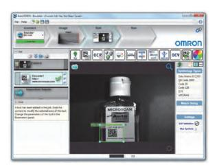
AutoVISION<sup>®</sup> is the easiest machine vision software available for basic to mid-range vision applications. Process and manufacturing engineers no longer need to become experts in machine vision in order to successfully deploy a system that meets their traceability, inspection and quality control needs.
