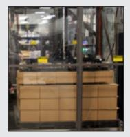
The process repeats until the load is completed, including adding a sheet to the top of the load.
