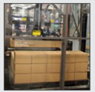
Product is received on the Infeed Conveyor at a 40" elevation. Product conveys to a stop and the Gantry lowers in position over the product on the conveyor.
